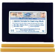
Kemdent inlay casting wax is a blend of paraffin waxes with beeswax and gum damar to give a tough, smooth wax resistant to flaking and cracking. Used for waxing up acrylic crowns and for the diagnostic wax-up of crowns, It enables an accurate fit to the prepared cavity. Available in medium hard and hard.
